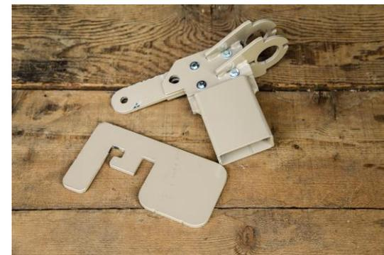
Assembly of the bracket takes only minutes. Simply remove your A-DAP bracket from your current target. The gussets will slide around the bracket as shown above. Slide the four bolts through the holes and ensure that you have the lock nuts fastened very tight so they do not come loose during use. The above picture shows the bracket assembled.
