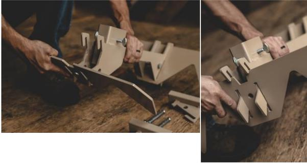
The rear shield simply slides into place, just like the front shield. You will notice that on both the front and the back there are holes for the clevis pins. These pins keep the shields onto the center sections so that you can move your assembled base around without it falling apart. There is also a spot for a 1/2" Grade 8 carriage bolt on the front shield. This offers a protective barrier in the square hole so bullets cannot easily pass through the hole. See below.
