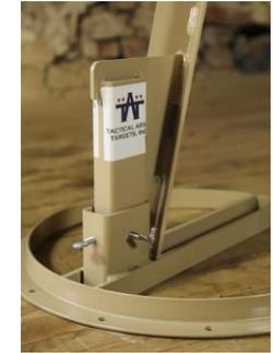
First, place the round base onto a level, flat area of ground. Then, with the help of a partner, slide the upper angle into the bottom tube as shown above. Then begin tightening the thumb screws on the side and back of the tube. You may need to rock the upright side to side while tightening the screws. Please be sure the screws are adequately tightened to ensure minimal movement of the target system.
