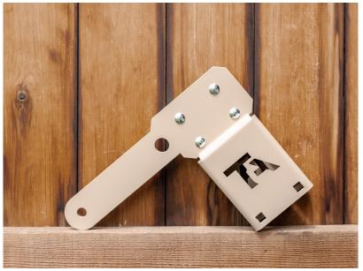
Upon receiving your new Gen 5 A-DAP Top Bracket you will see that it is TWO HALVES that are bolted together with (4) <sup>1</sup>/<sub>4</sub>" Carriage bolts and locking nuts. We utilize carriage bolts for ease of install and removal. For your convenience each A-DAP top bracket is PRE-ASSEMBLED prior to shipping.
