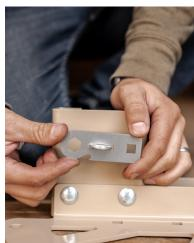
The 2X4 base tube has a tapped hole on the front and back. This is so the tube can be installed in any left/right orientation. It is NOT recommended to put the thumb screw on the FRONT of the tube.
