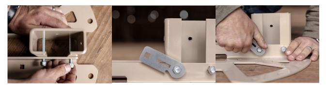
Step Four: If you desire to use cardboard targets with your base, install the paper holders. A left and right paper holder are included with each base. Use the included carriage bolts and install the bolts from the BOTTOM of the base. Then place each paper holder over the bolts. Then install the washers, last install the wing nuts hand tight. Thread locker is not required on this part and is not recommended UNLESS you permanently desire your paper holders to be mounted to your base.
