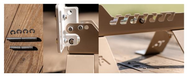
Step Nine: Re-installing the locking clevis and cotter pin. You'll notice two holes in the target base that retained your target in the locking position. After set up, re install the clevis pin through the holes in the target base to keep the target from camming over and staying in the downward position. This limits the rearward travel of the target plate, which aids in adding some bounce and over-all returning to upward position during heavy usage.
