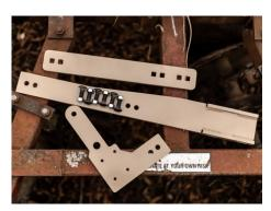
For installation use either a ¾" Socket or a ¾" Open Wrench. The carriage bolt squares will prevent the bolts from spinning during tightening. Hand tighten ALL bolts and nuts. Always check for tightness prior to training on each range day. Orientation of the center splice plate does NOT matter. Mount to either the left or right sides of the top and bottom sections.
