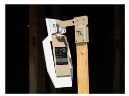
The first step will be installing the paddle. It simply fits over the bent gusset as shown. Then install the A-DAP Top Bracket or Armored Post. We ship the clevis pin with TWO Aluminum Bushings. Insert the Pin through one side of the bent bracket, then add a bushing, then the top bracket, and one more busing on the opposite side before pushing the pin through the other side of the bent bracket. We then include a hairpin clip to keep the pin in place. See above picture.
