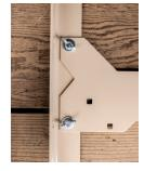
After the center is placed into the correct position, install a washer, then a wing nut onto EACH carriage bolt. See the image to the left. Do this to BOTH sides of the cardboard base.
