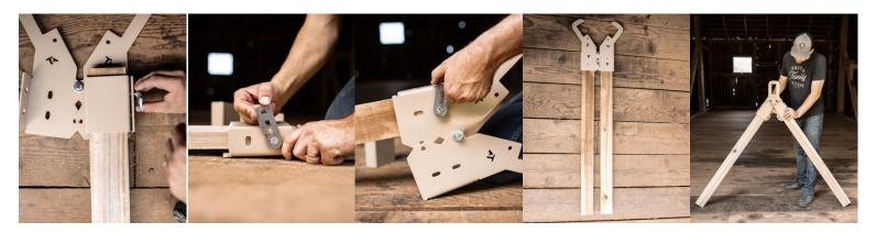
Each tube bracket has a 3/8-16 tapped hole on one of the long sides and one of the short sides of the bracket. There are no "right and left" tube brackets, they are identical. For this reason, they will be oriented opposite in the left and right bracket. This is why there are vertical slots in the left and right "A Frame" Brackets.
