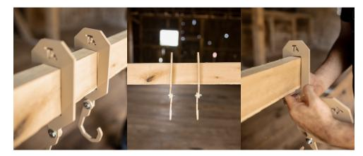
The included hooks are pre-assembled. Occasionally during use you should check bolt tightness and bolt wear and tear. If the bolt shows signs of wear, replace it. When tightening the bolt please NEVER over tighten. It should be JUST tight enough to have full thread engagement with the locking nut, but loose enough that it pivots freely. Install with hook openings facing the direction of shooting to ensure gongs stay in place.
