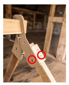
Take careful notice of the picture on the left and the picture on the right. You will notice the orientation of the bolts. One of the tubes on each A Frame will utilize the topmost set of holes, then the opposite will use the bottom side. This is designed in this fashion so as to not need to produce left and right tube steel brackets.
