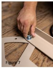
3.) If you desire to install paper holders, simply place the paper holders over the front four bolts as shown here:
