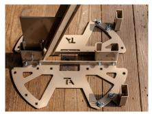
First, place the round base onto a level, flat area of ground. Then, with the help of a partner, slide the upper angle into the bottom tube as shown above. Then begin tightening the thumb screws on the side and back of the tube. You may need to rock the upright side to side while tightening the screws. Please be sure the screws are adequately tightened to ensure minimal movement of the target system.
