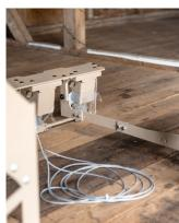
There are two pieces of hardware required for each post to be installed. There is (one) clevis pin and clip that goes into the hole closest to the shield. Then there is a ¾" structural bolt that goes into the larger hole. We ship the bolts and pins along with the skid. Install the clevis pin, then install the ¾" Bolt. Make sure the clevis pin clip is in place and then tighten the ¾" nut onto the bolt to approximately 20 ft/lbs. It just needs to be snug. There is no need to over torque it.
