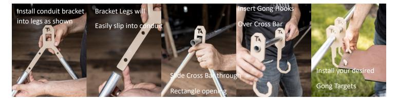
Take the conduit leg bracket for one site, install the two pieces of conduit over the legs. If you purchased the correct conduit, the bracket legs will slip freely into the conduit. This creates an "A" Frame that becomes rigid when completely assembled. Next, slide the cross bar through the square opening. This square opening creates a wedge when the legs are angled outward.
