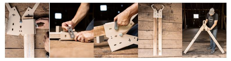
Each tube bracket has a 3/8-16 tapped hole on one of the long sides and one of the short sides of the bracket. There are no "right and left" tube brackets, they are identical. For this reason, they will be oriented opposite in the left and right bracket. This is why there are vertical slots in the left and right "A Frame" Brackets.
