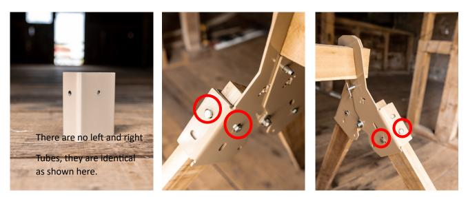
Take careful notice of the picture on the left and the picture on the right. You will notice the orientation of the bolts. One of the tubes on each A Frame will utilize the topmost set of holes, then the opposite will use the bottom side. This is designed in this fashion so as to not need to produce left and right tube steel brackets.
